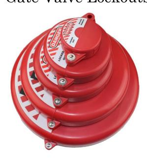
Our Gate Valve Lockout devices have a clamshell design, completely encompassing a gate valve. Once locked, using a padlock, hasp or security seal, the clamshell rotates freely around the hand wheel, preventing it from being turned. Available in 6 sizes to fit standard gate valves.
